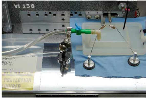
FIG. 6—Valley instruments rotary beam spin fatigue tester.
